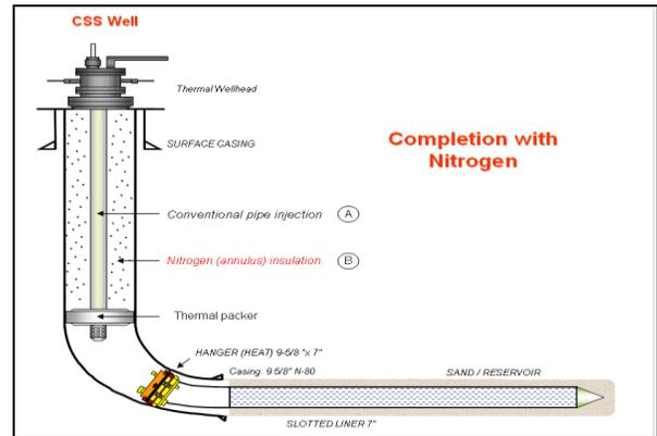
**Figure 2:** Well Completion with Conventional Tubing and Trapped Nitrogen in the Casing-Tubing Annulus.
