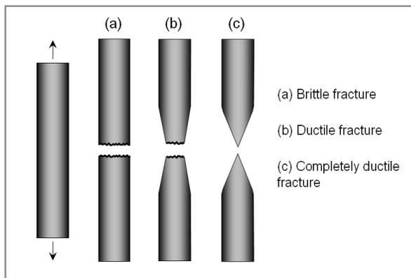
**Figure 4:** Schematics of Round Metal Bars After Tensile Testing
