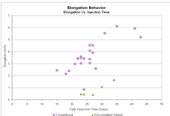
**Figure 10:** Steam Injection Time vs Wellhead Elongation
