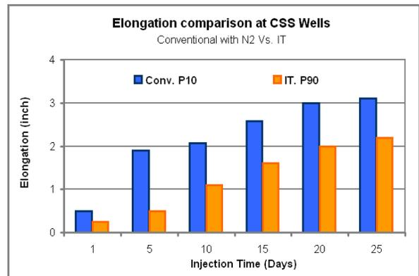
**Figure 9:** Elongation Percentile for Wells using Conventional Tubing (P10) and Insulated Tubing (P90)
