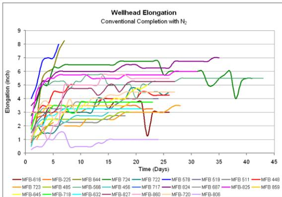
**Figure 7:** Wellhead Elongation using Conventional Completion
