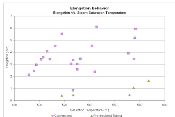
**Figure 11:** Steam Saturation Temperature vs Wellhead Elongation
