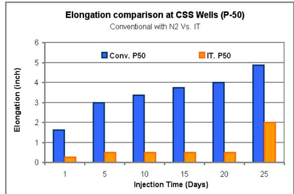
**Figure 15:** Elongation with respect to Injection Time (P50 Case)
