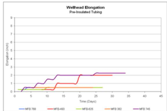
**Figure 8:** Wellhead Elongation using Insulated Tubing
