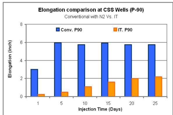
**Figure 16:** Elongation with respect to Injection Time (P90 Case)
