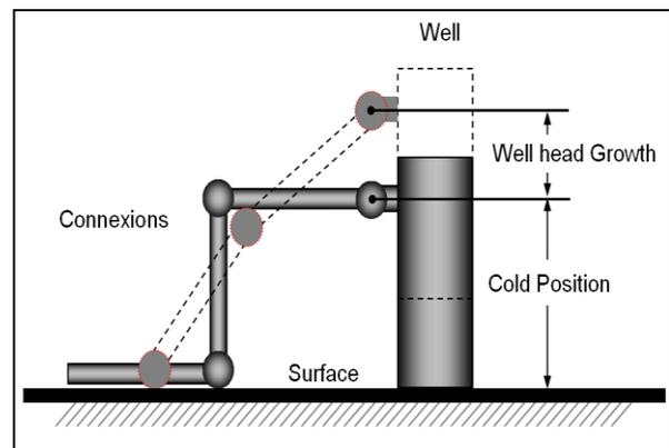
**Figure 6:** Wellhead Elongation Schematic
