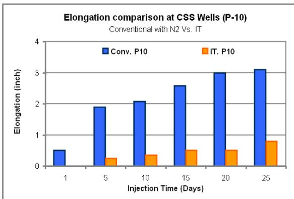
**Figure 14:** Elongation with respect to Injection Time (P10 Case)
