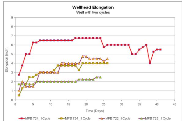
**Figure 13:** Wellhead Elongation in Wells with Two Steam Injection Cycles
