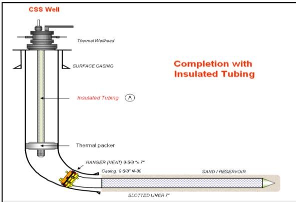
**Figure 3:** Well Completion using Insulated Tubing
