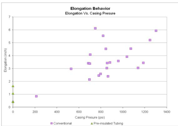
**Figure 12:** Casing Pressure vs Wellhead Elongation
