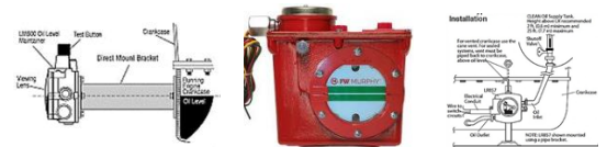
Fig. 13. Oil Lubrication System.
