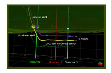
In this phase, the magnetic guide tool is used, which helps to more accurately position the injection well, reducing errors in the survey.
