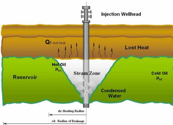
Figure # 4. Steam injection stage. Vertical well.
