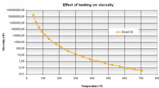
Figure # 6. Effect of temperature on viscosity.
