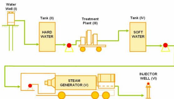
Figure # 1. Steam generation process
