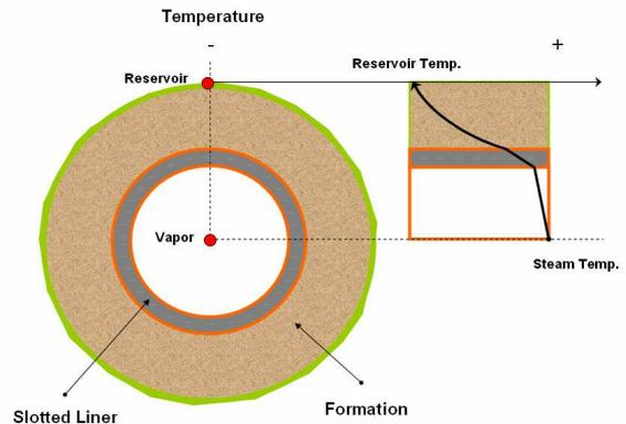
Figure # 5. Soaking time in a horizontal well
