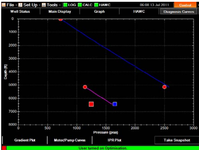
Figure 6. Initial system calibration; calculated gradients are correlated with the red points, which are the pressure measured points sensed by the gauges.
