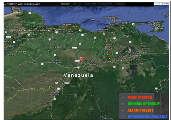
Figure 7. Screen of Well Status, Using a Color Code on a Map
