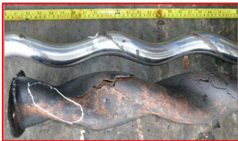
Fig. 6. Discharge section of the all metal PCP that failed in the well MFB-722.
